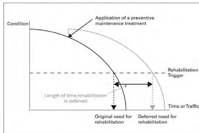
Figure 8D: Preventative Maintenance Treatments Slow the Rate of Pavement Deterioration<sup>48</sup>
